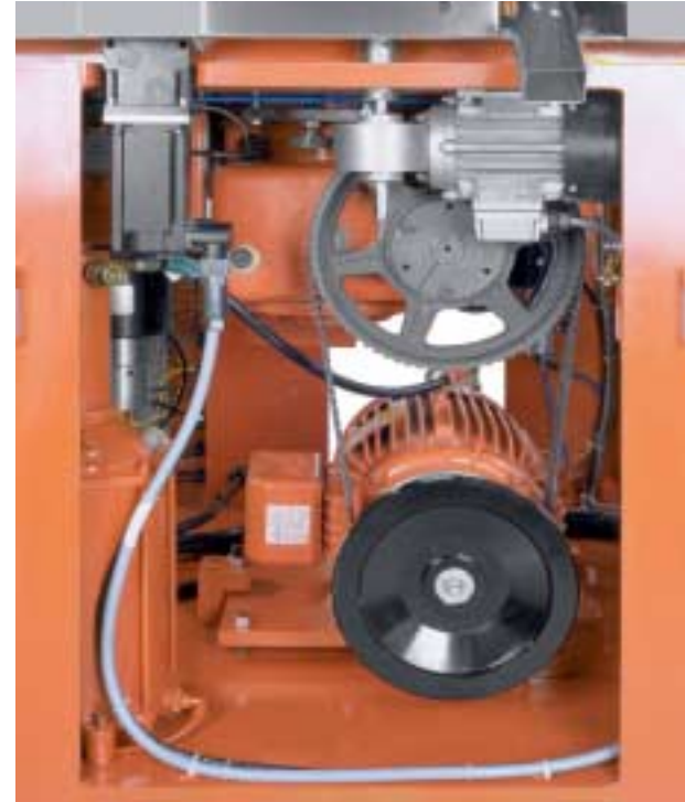
Drive Motor & Gearbox, Feeder Motor, and Overload System
